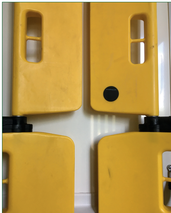
Figure 2. For consistency, stickers at the same place on scoop stretchers provided a target for thermometers
